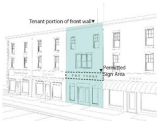
Figure 14-3 Multi-Tenant Building Sign Measurement
